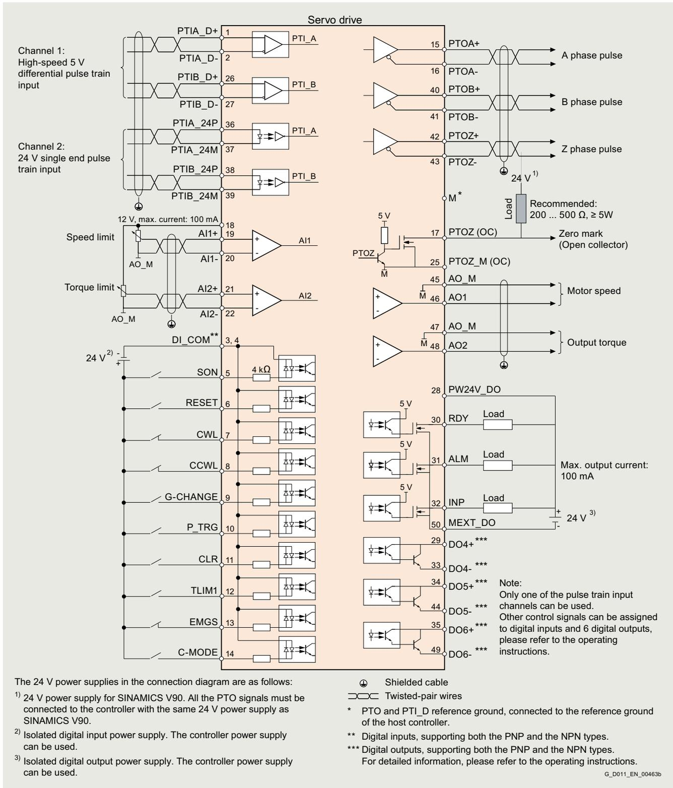
Standard wiring for pulse train input (PTI) position control mode (for detailed information and connection diagram for other control modes, please refer to the operating instructions). The diagram is given as a reference for selecting the drive type.
