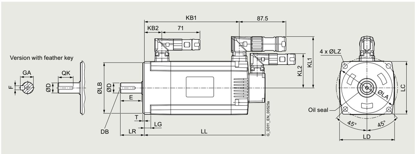
SIMOTICS S-1FL6 Low Inertia servomotor, shaft height 50
