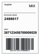
Example of a MIX pallet, carrying multiple products on a single pallet (A6 or A5 size)
